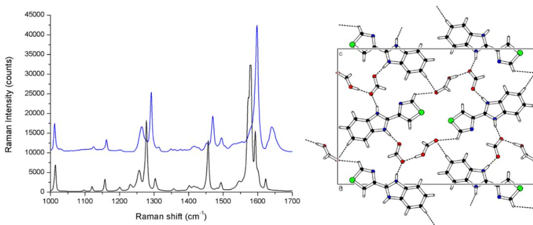
Figure 1 – Raman spectra of the thiabendazole (black) and of the new TBZ-formic acid solvate (blue) [left], and molecular packing of the TBZ-formic acid solvate [right].
