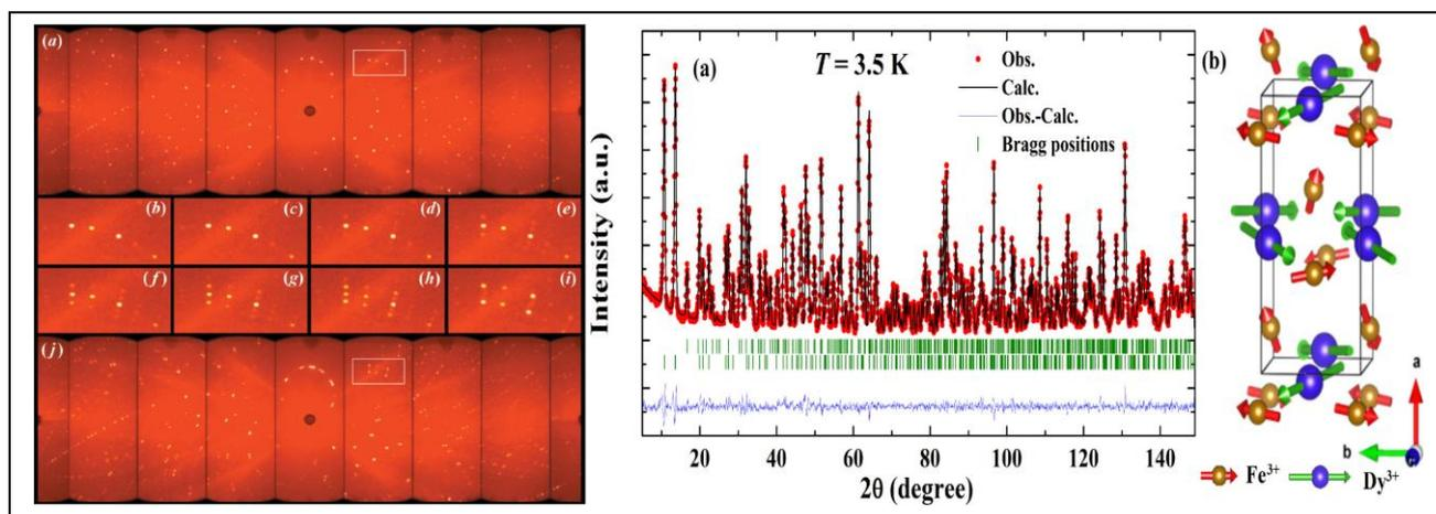
**Figure:** (left) Series of snapshots at different temperatures taken on CYCLOPS for studying the phase transition on the compound  $[\text{CH}_3\text{NH}_3][\text{Co}(\text{COOH})_3]_1$  (right) Refinement of the crystal and magnetic structure of the compound  $\text{DyFeWO}_6$  using symmetry modes within Shubnikov magnetic space groups<sup>2</sup>.
