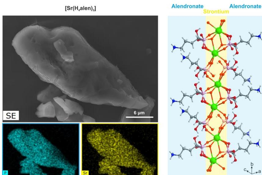
**Figure 1:** (Left) SEM images of  $[\text{Sr}(\text{H}_4\text{alen})_2]$  and EDS mapping showing the uniform distribution of P from alendronate linker and Sr metallic centres. (Right) Structural representation of the bio-MOF, highlighting its two components.
