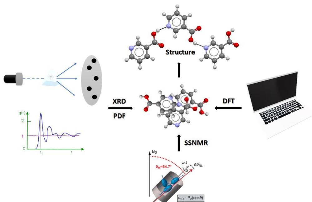
**Figure 1:** Schematic representation of the multi-faceted approach for the characterization of small drug molecules.
