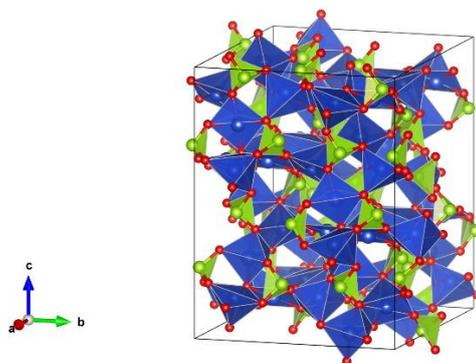
**Figure 1:** Structure of the monoclinic polymorph of  $\text{Cu}_4\text{O}(\text{SeO}_3)_3$ , depicting the coordination polyhedral of the Cu atoms in blue and those of Se atoms in green.
