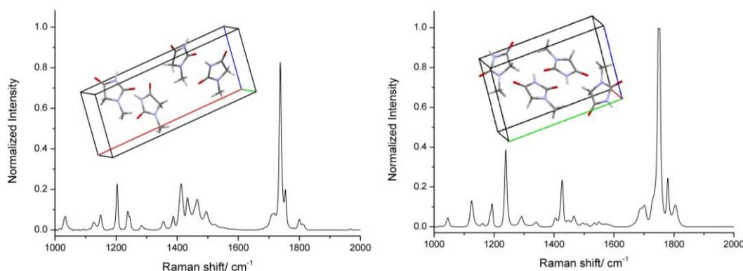
**Figure 1:** Molecular packing and characteristic Raman signature for the polymorphs I (left) and II (right) of 1-MH.
