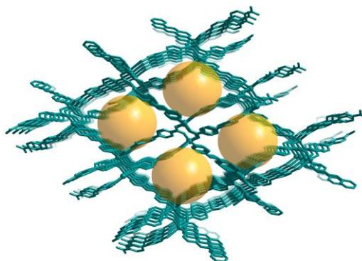
**Figure 1:** Schematic representation of the crystalline structure of the FMOF, Zn<sub>2</sub>(bpdC)<sub>2</sub>(bpee).
