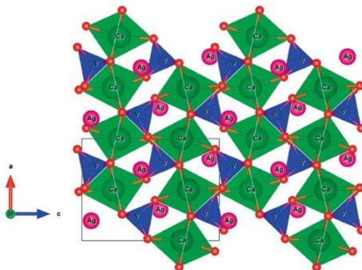
**Figure 1:** Crystal structure of AgCaVO<sub>4</sub> solved from Aeris data.
