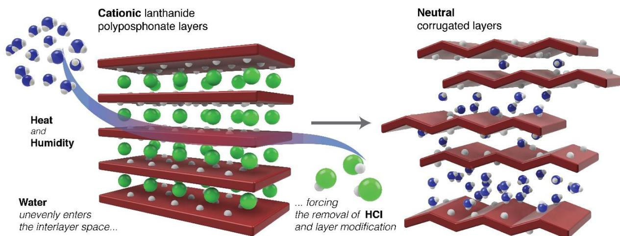
Figure 1 - Schematic representation of the structural transformation of  $[Gd(H_4nmp)(H_2O)_2]Cl \cdot 2H_2O$  (**1**, left) into  $[Gd_2(H_3nmp)_2] \cdot xH_2O$  (**2**, right) ( $x = 1$  to 4) at high temperature and humidity.
