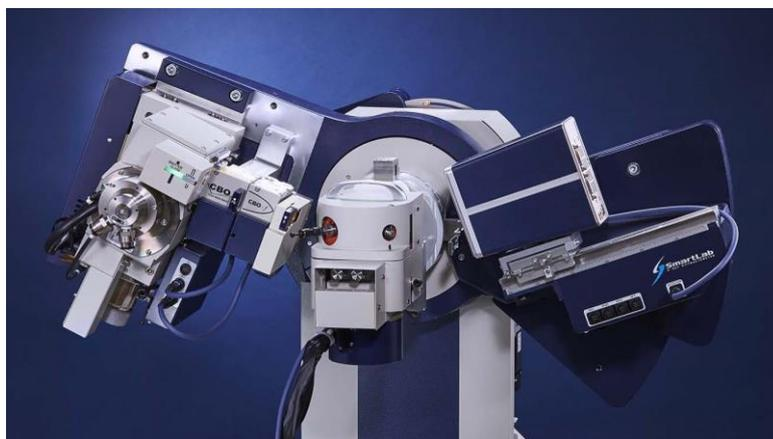
**Figure 1:** SmartLab system with XRD-DSC chamber
