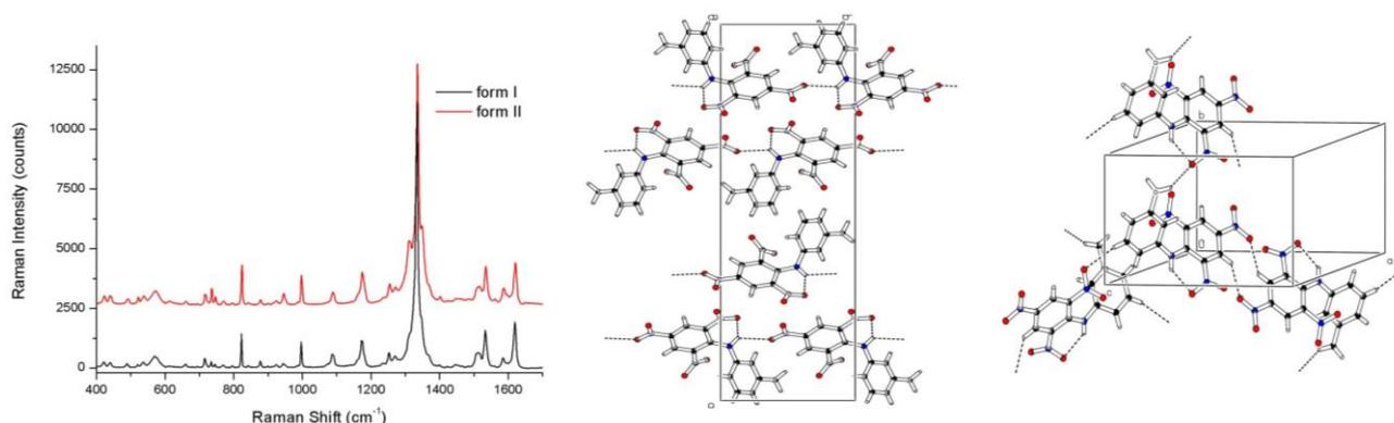
**Figure 2:** Raman spectra of two different polymorphic forms of 2,4,6-trinitro-*N*-(*m*-tolyl)aniline (*left*) and the corresponding molecular packing (form I, *middle*; form II, *right*).
