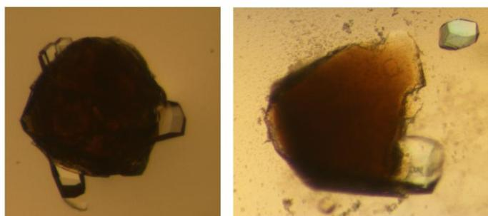
**Figure 1:** Lysozyme crystals grow abundantly at the surface of millimeter-size Tb-mesoMOF crystals
